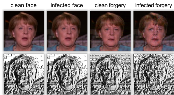
Figure 6: Some visual examples of defending against face reenactment ( \epsilon = 0.02 ). The bottom row is the pertinent LBP features of the top row, and the forgeries are generated from the same expression landmark.
